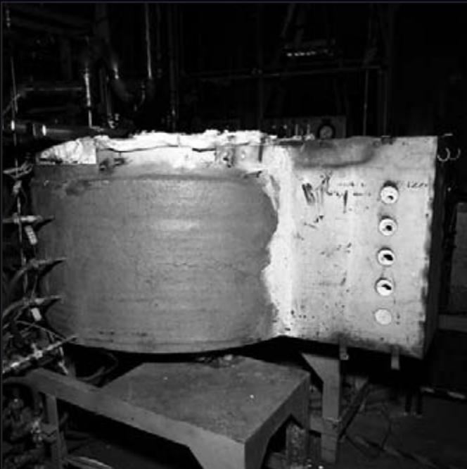
*Jet Test for Slurry Tank*
