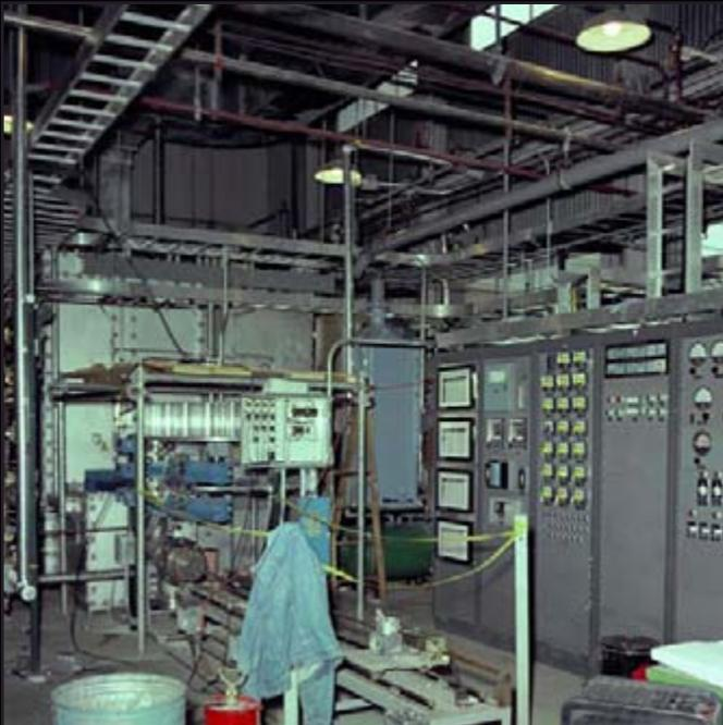
*Control Panels for the Melter System*
